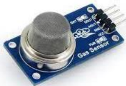
Gambar 7. Sensor Gas MQ7 (Sumber: https://ae01.alicdn.com/ )
